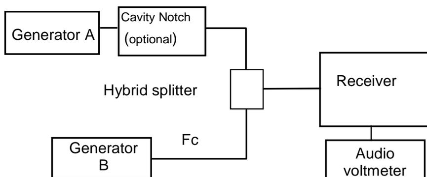
**Figure 4: Measurement arrangement**
