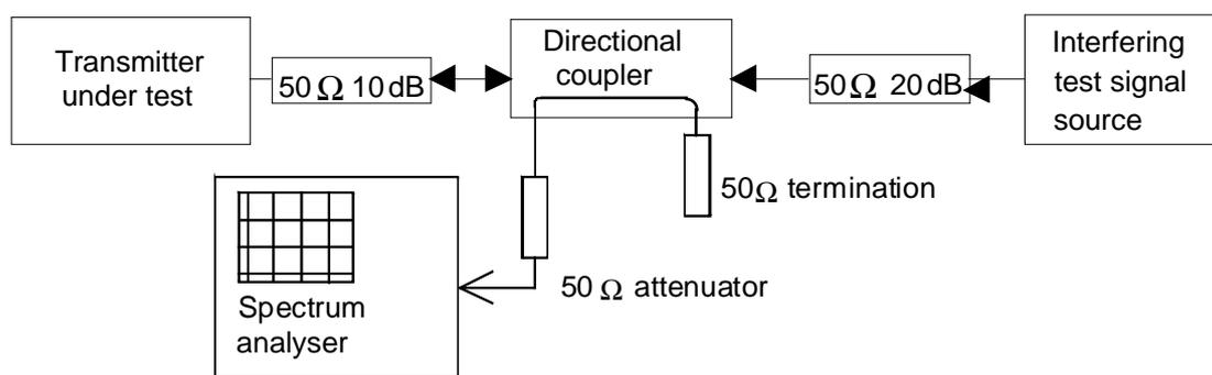
**Figure 2: Measurement arrangement**
